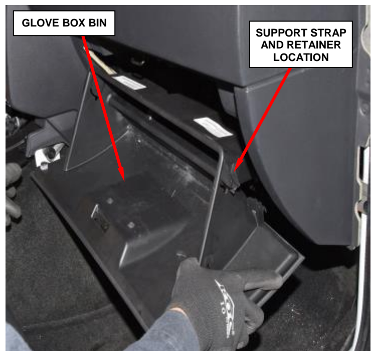
Figure 94 – Glove Box Bin
