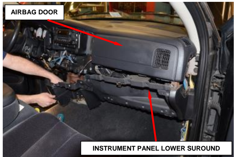
Figure 11 – Instrument Panel Lower Surround
