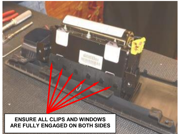
Figure 29 – Airbag Cover and Airbag Module
