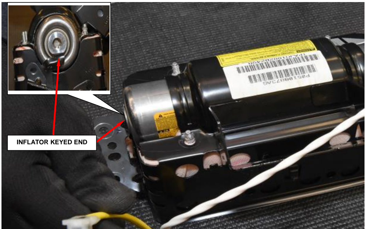
Figure 109 – Inflator End Position
